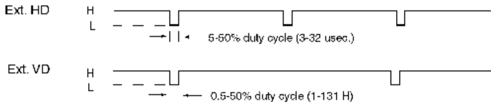
Figure 10. External Synchronization and Gen-lock Timing
