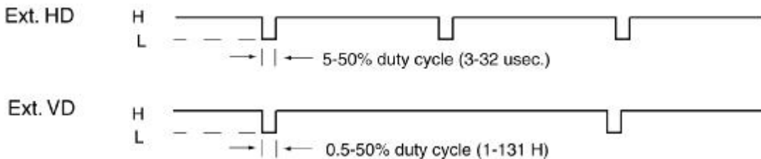
Figure 11. External Synchronization and Gen-lock Timing
