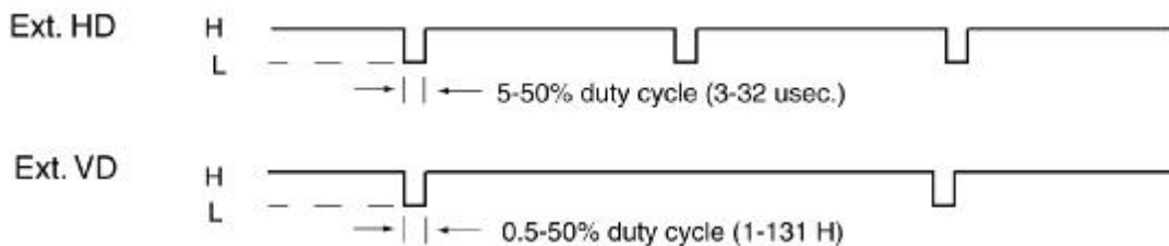
Figure 11. External Synchronization and Gen-lock Timing
