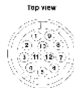
Figure 2. 12-Pin Hirose Connector
