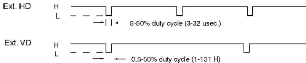
Figure 10. External Synchronization and Gen-lock Timing
