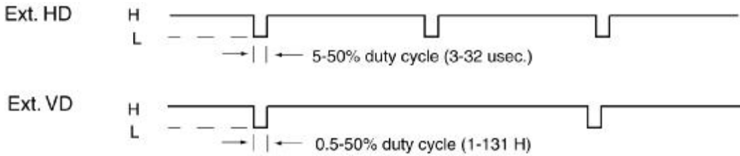
Figure 7. External Synchronization and Gen-lock Timing
