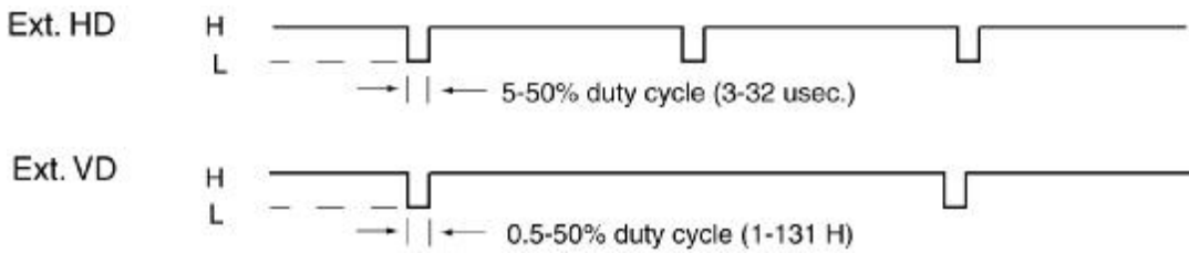
Figure 7. External Synchronization and Gen-lock Timing
